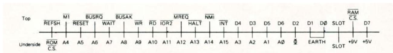
The RAM C.S. and ROM C.S. lines on the ZX81, and the WE on the Ace, don't need connecting.
