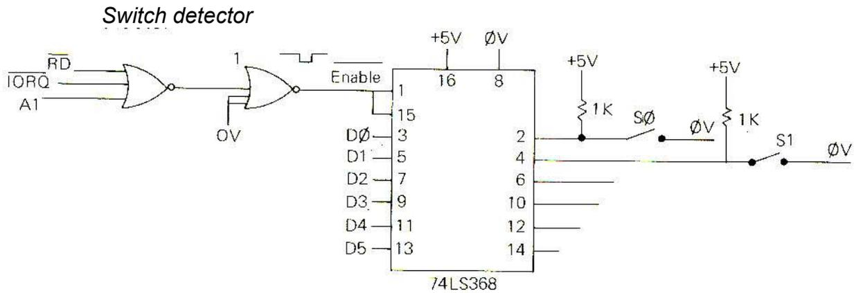
Switches S2 to S5 are similar to S0 and S1, each with a 1K resistor, and are connected to pins 6, 10, 12 and 14.
